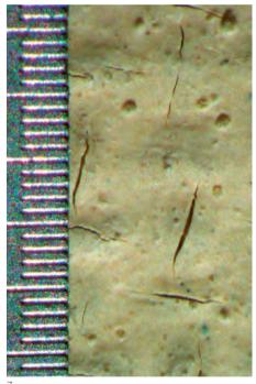
Ill. 10 The sample surface: the red lines indicate micro-fissures in the layer.
